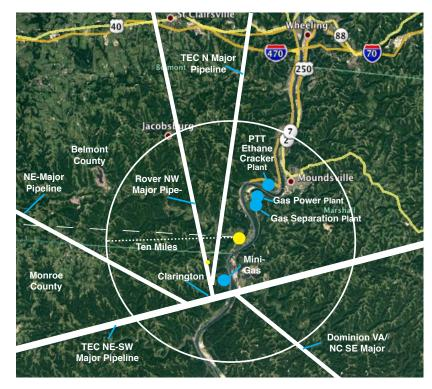
Figure 4. Powhatan Point Location and Area Major Gas Intersection Pipeline, Power Plant and Mini-Cracker Projects
